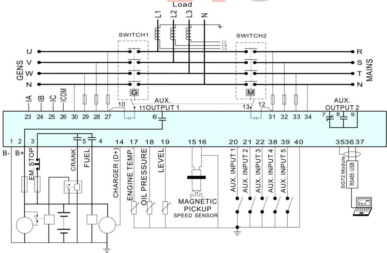
**Fig.6 - HGM6120NC Typical Application Diagram**
